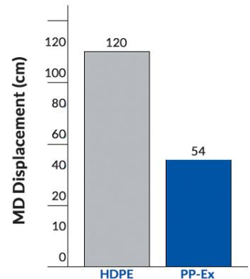
MD displacement per 100m length of geomembrane when exposed to a 50°C temperature change (20°C - 70°C)
